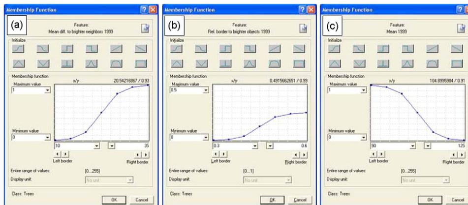
Fig. 4. Fuzzy membership functions used to classify ‘edge forest’ (a) high mean difference to brighter neighbors, (b) high relative border to brighter objects, and (c) low mean brightness.
