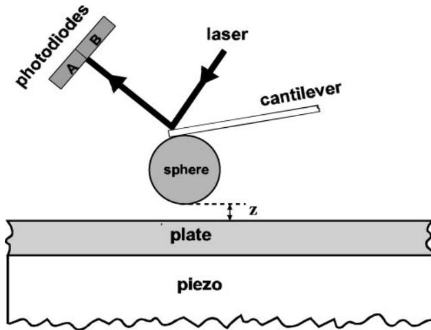
**Figure 9** Schematic diagram of the Casimir-force apparatus used in Reference (165).
