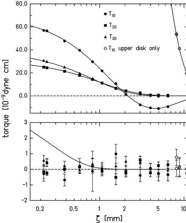
**Figure 2** *Top:* Torques measured in the first experiment of Hoyle et al. as a function of pendulum/attraction separation. Open circles are data taken with the lower attractor disk removed and show the effect of uncanceled gravity. Smooth curves show the Newtonian fit. *Bottom:* Residuals for the Newtonian fit. The solid curve shows the expected residual for a Yukawa force with  $\alpha = 3$  and  $\lambda = 250 \mu\text{m}$ .
