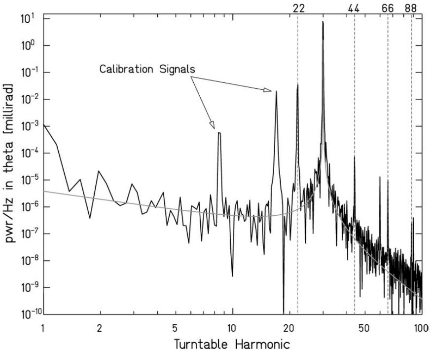
**Figure 3** Spectral density of the torque signal in the 22-fold symmetric experiment of the Eöt-Wash group. The peaks at  $8.5$  and  $17\omega$  are gravitational calibrations; the fundamental and first three overtones of the short-range signal are at  $22$ ,  $44$ ,  $66$ , and  $88\omega$ . The smooth curve shows the thermal noise computed using Equation 33.
